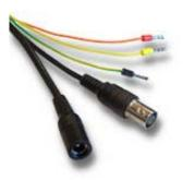
BNC video output - At the BNC female bayonet connecting the video cable that then leads to the DVR typically through RG59 type coaxial cable and BNC connector. You can also use twisted pair cables with balun converters.
